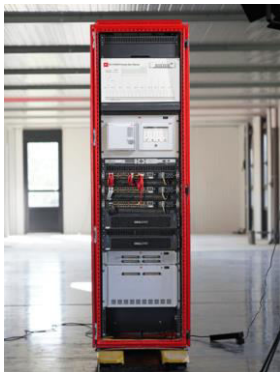
Fig 9. The stand for modeling the Typhoon HIL platform
