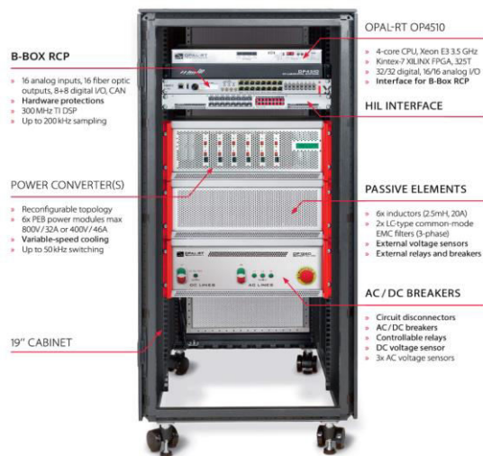
Fig 7. The stand for modeling the Opal-Rt platform
