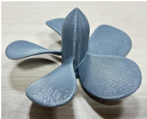
Figure 4. 3D printed part Propeller – FDM technology, material PETG
