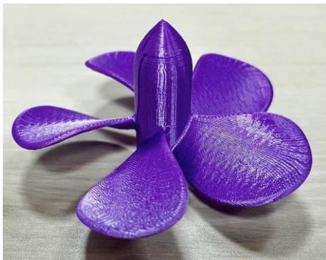
Figure 5. 3D printed part Propeller – FDM technology, material SILK
