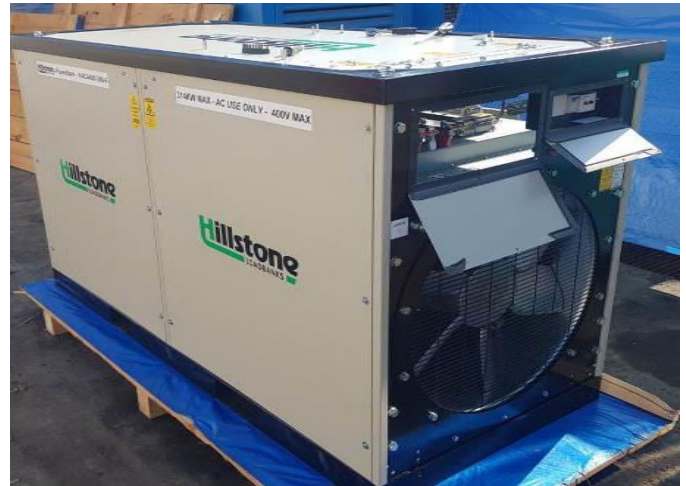
Figure 3. Hillstone load bank 3 phase AC, 400V, 319 kW
