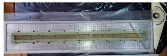
Fig. 1 A perforated plate with a gasket
