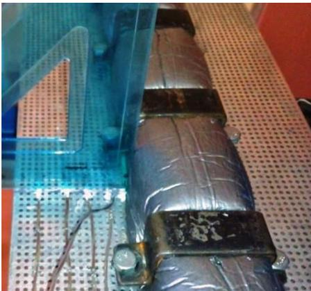
Fig. 3 Thermocouples positions on a perforated plate
