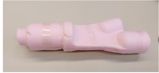
Figure 8. Styrodur model made on a CNC mill
