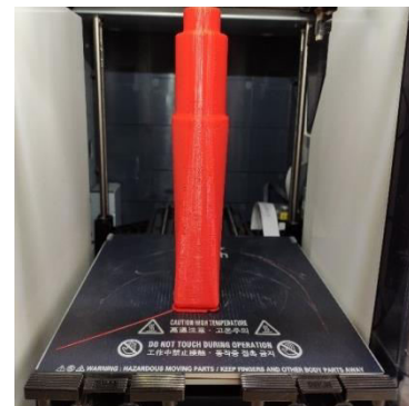
Figure 4. Manufacturing of sleeve model on a 3D printer
