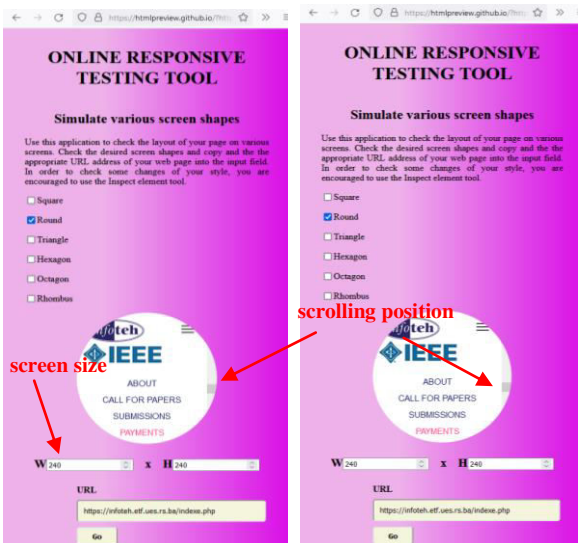
Figure 9. Opened sticky menu viewed in Responsive testing tool, [30]-[32] on a round shaped screen with dimensions 240x240px
