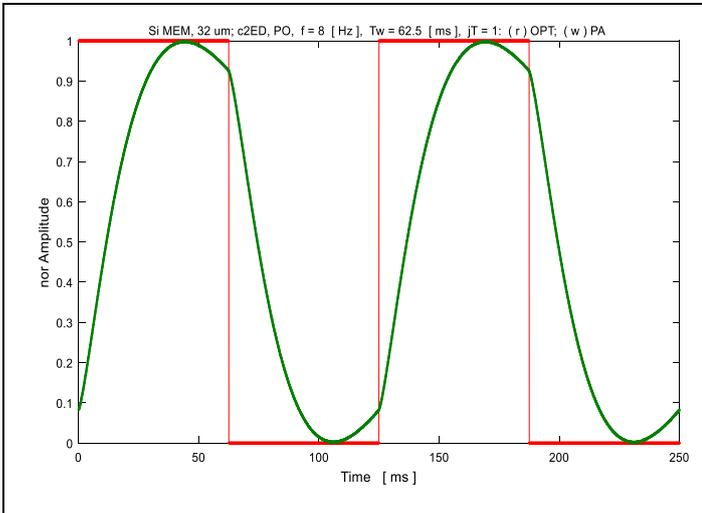
Fig. 2. Normalized and synchronized optical and PA signals (two periods) for a micromechanical structure - Si membrane 32  $\mu\text{m}$  thick (Si chip with frame 5 x 5 mm and square membrane 3 x 3 mm). (red) optical signal; (green) PA signal.
