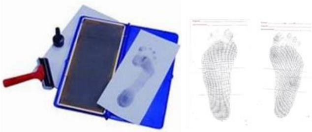
Figure 2. Ink based footprint printer [1], [2]
