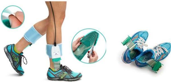
Figure 6. An in-shoe plantar pressure measurement [15]
