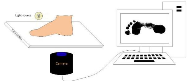
Figure 3. Pedobarographic system based on application of one camera
