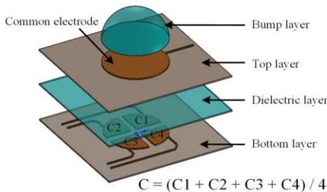
Figure 8. Capacitive sensor construction [18]
