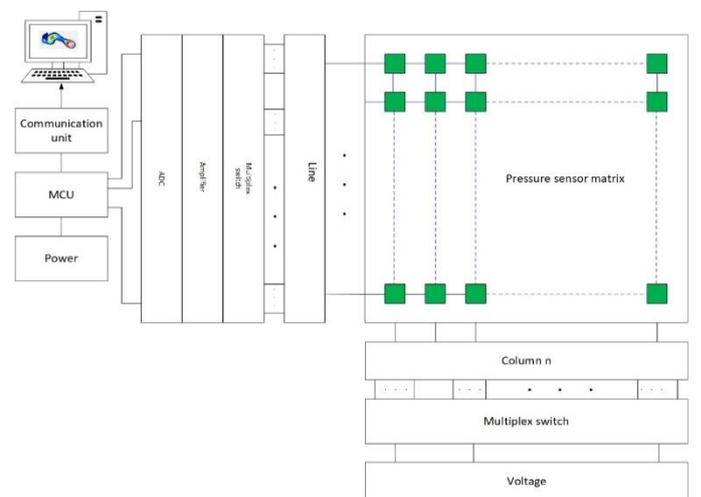
Figure 4. Plantar pressure distribution platform data acquisition system
