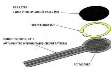
Figure 9. Force sensing resistor [19]
