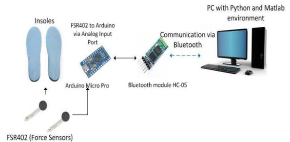
Figure 11. Example of hardware system for foot plantar sensor acquisition [2]
