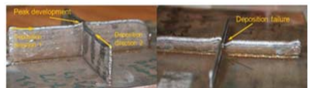
Slika 3. Camber and sag in WAAM products [1]
