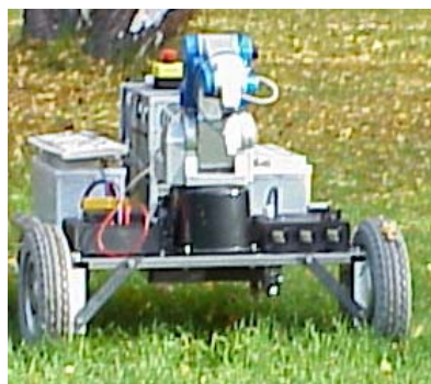
Fig. 2. Prototype of the mobile platform with articulated robot without ultrasonic measurement lay out
