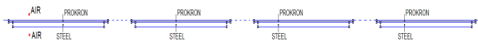
Figure 6. 2D Geometry of busbars in the sill of the sluice and assigned materials
