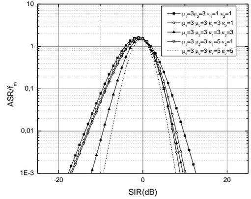
Figure 1. Normalized ASR of an AFC in  $k$ - $\mu$  multipath fading environment for different values of  $k_1$  and  $k_2$  and constant value of parameters  $\mu_1$  and  $\mu_2$ .
