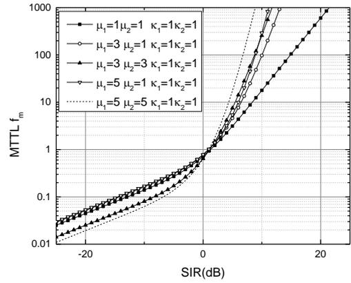
Figure 4. The MTLL of an AFC in  $k$ - $\mu$  multipath fading environment for constant values of  $k_1$  and  $k_2$  and different values of parameters  $\mu_1$  and  $\mu_2$ .
