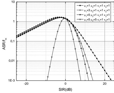
Figure 2. Normalized ASR of an AFC in  $k$ - $\mu$  multipath fading environment for constant values of  $k_1$  and  $k_2$  and different values of parameters  $\mu_1$  and  $\mu_2$ .
