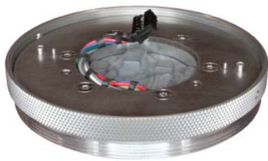
Fig. 5. Barrett 6-axis force / torque sensor is completely independent device that significantly improves the properties of WAM hands.
