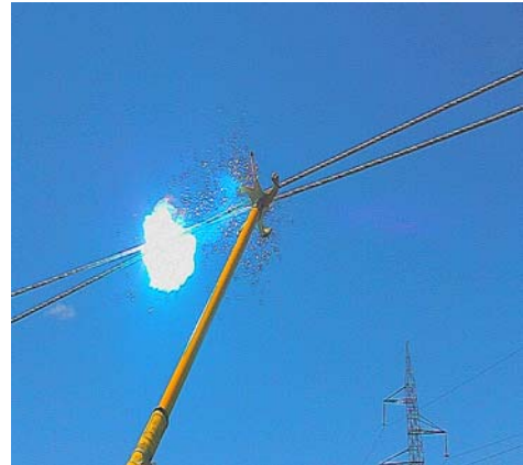
Figure 1. Sparks produced by conductor clashing (short circuit) experiment
