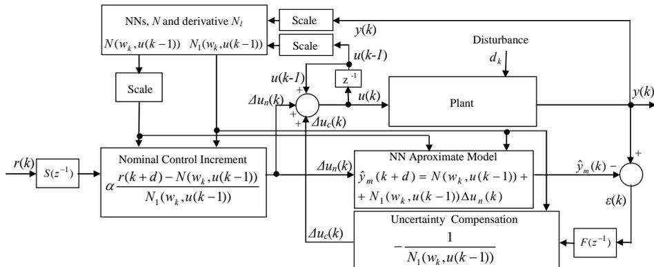
Figure 3. The conceptual structure of the modified AIMNC
