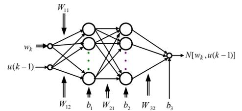
Figure 2. Double-layered MLP structure
