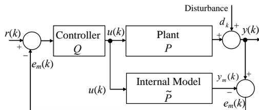
Figure 1. The IMC structure
