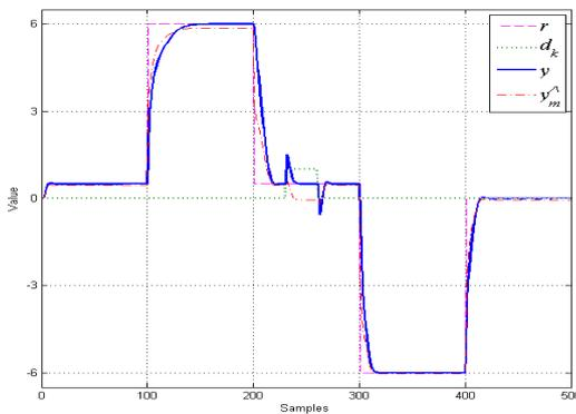
Figure 4. Reference  $r$ , disturbance  $d_k$ , system  $y$  and model  $\hat{y}_m$  outputs
