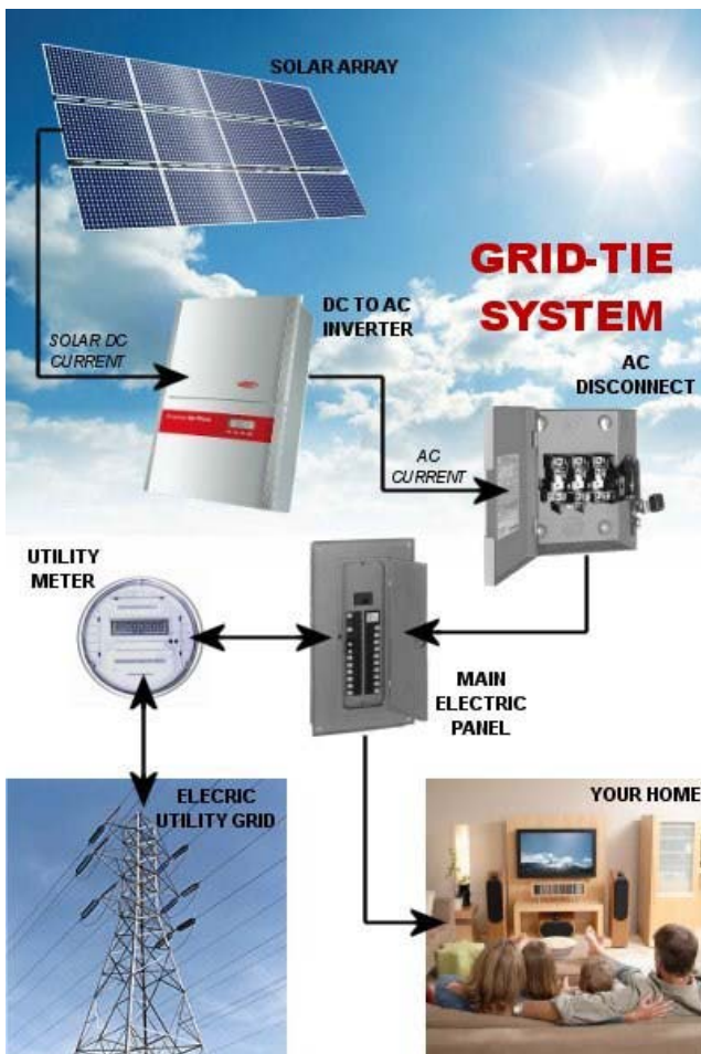
Fig. 3 Grid tied solar power system [11]
