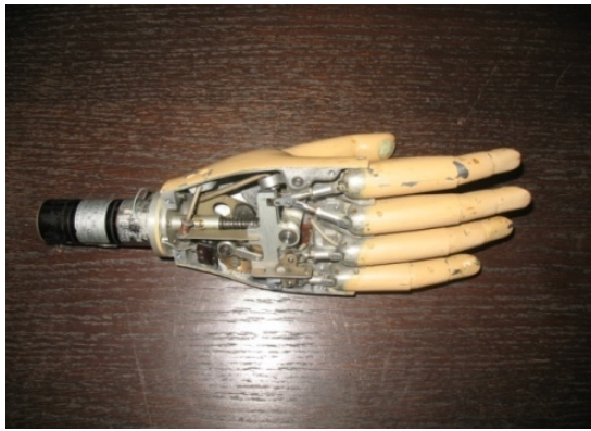
Figure 3. Lever mechanism in Belgrade hand
