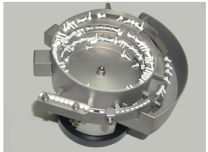
Figure 2. Vibratory bowl feeder with electro-mechanical drive
