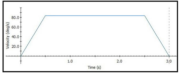
Figure 6. The velocity diagram of the AC servo motor for the C-arm rotation around the support plate
