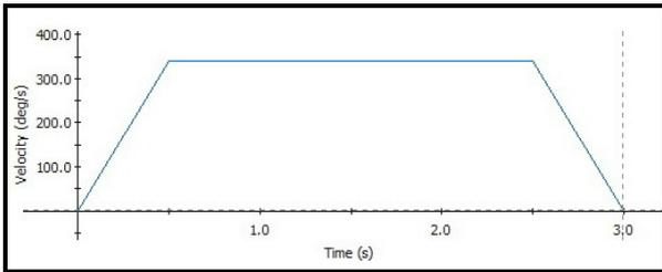
Figure 9. The velocity diagram of the drive for the C-arc rotation around the vertical plane for 30°
