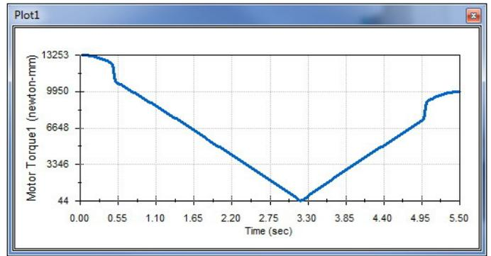
Figure 7. The torque diagram of the AC servo motor for the C-arm rotation around the support plate
