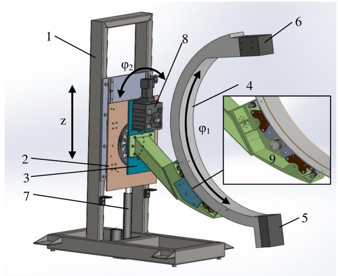
Figure 1. The new Radiography Positioner System
