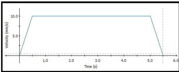
Figure 3. The velocity diagram of the linear actuator for the C-arm assembly linear motion
