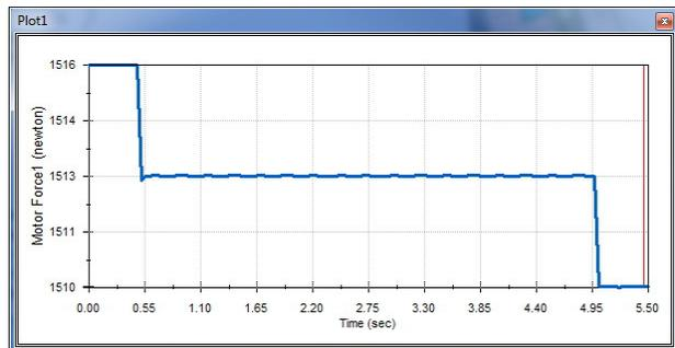
Figure 4. The force diagram of the linear actuator for the C-arm assembly linear motion
