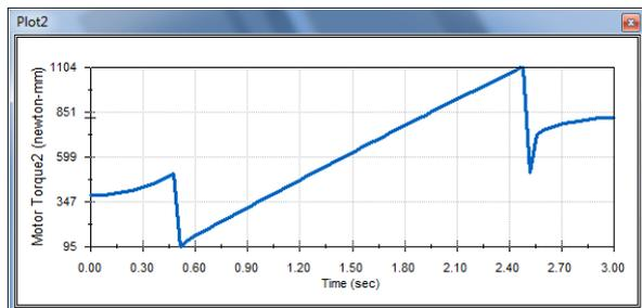
Figure 12. The torque diagram of the drive for the C-arc rotation around the horizontal plane for 30°
