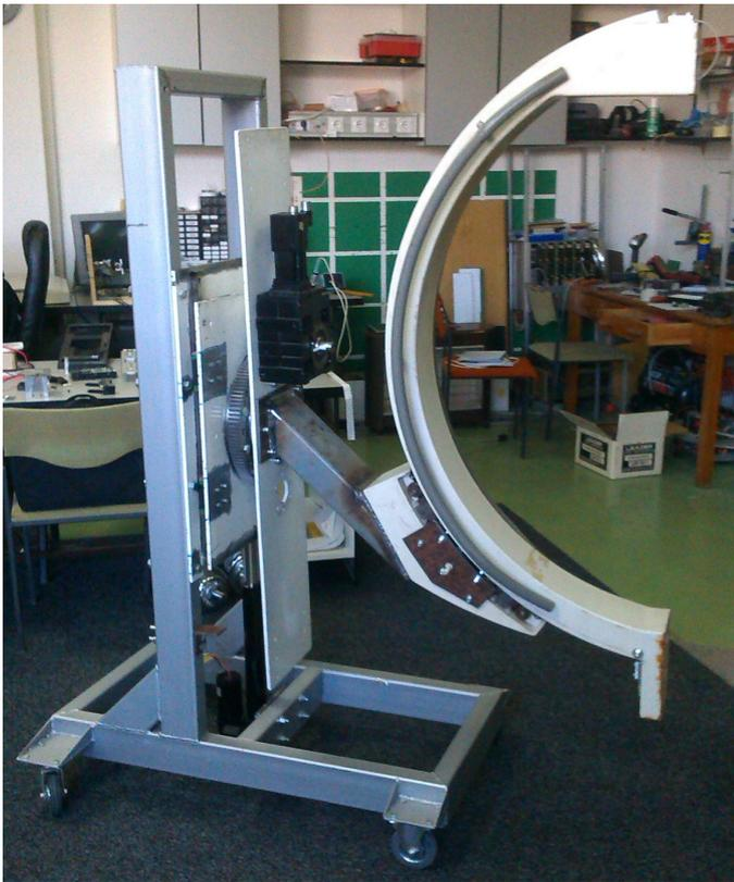
Figure 16. The prototype of the developed Radiography Positioner System
