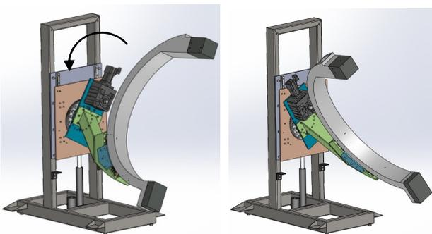
Figure 5. The analysis of the C-arm assembly rotation around the support plate
