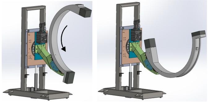
Figure 13. The analysis of the C-arc rotation from the vertical to horizontal position
