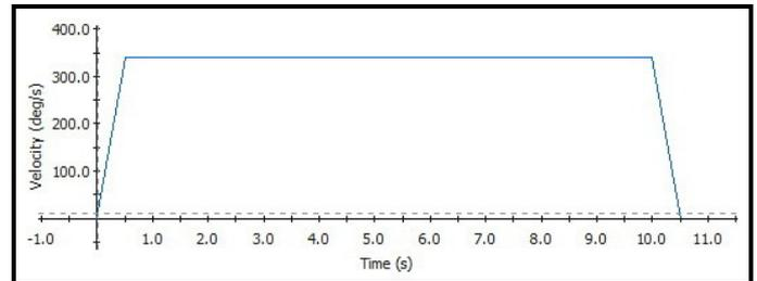
Figure 14. The velocity diagram of the drive for the C-arc rotation from the vertical to the horizontal position
