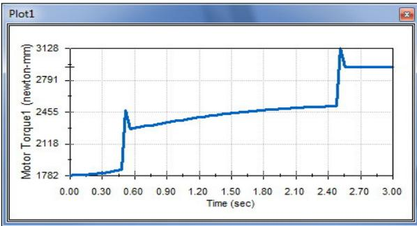
Figure 10. The torque diagram of the drive for the C-arc rotation around the vertical plane for 30°
