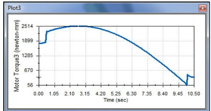
Figure 15. The torque diagram of the drive for the C-arc rotation from the vertical to the horizontal position
