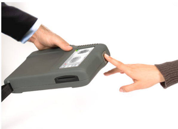
Figure 10. VDR-H is equipped with wireless or PMR modem and encryption functions. Thus, it can be used in the lines of cars at the border crossing, which reduces the queues and the waiting time. Alternatively, the train passengers can be checked while the train is still in motion.
