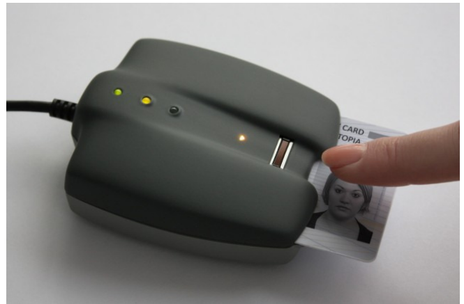
Figure 5: Vlatacom biometric access device is a smart card reader with integrated fingerprint scanner and security access module. The device allows the eID holder to authenticate him- or herself to e-Government servers, sign electronic documents and exchange confidential information by using his or her finger instead of the PIN code. The smart cards used with this device possess the "match-on-card" capability, performing the comparison of the scanned with the enrolled fingerprint on the chip. Otherwise, the risk of identity theft would have occurred as a result of the upload of the fingerprint to the computer.
