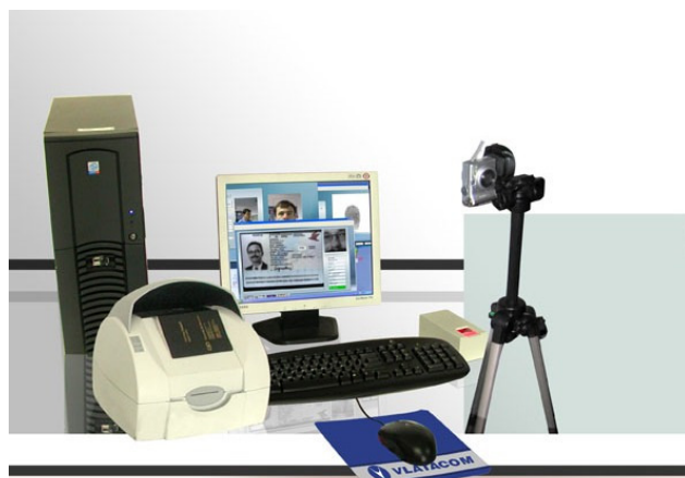
Figure 2: The acquisition equipment of different vendors controlled by Vlatacom enrolment application software. The passport scanner shown in the left-hand side is optional and serves for acquisition of demographic data from a previously issued ID document (either passport or ID card).
