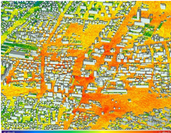
Fig. 2. 2D Electric field strength at frequency 900 MHz, 5m x 5m
