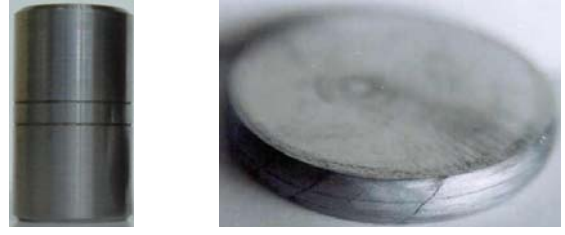
Figure 11 - Specimen with initial dimensions \varnothing 20 \times 25 mm before and after crash [3]
