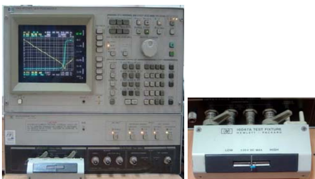
Slika 1. Analizator impedanse (Impedance/Gain - Phase Analyzer) HP 4149A i adapter 16047A
